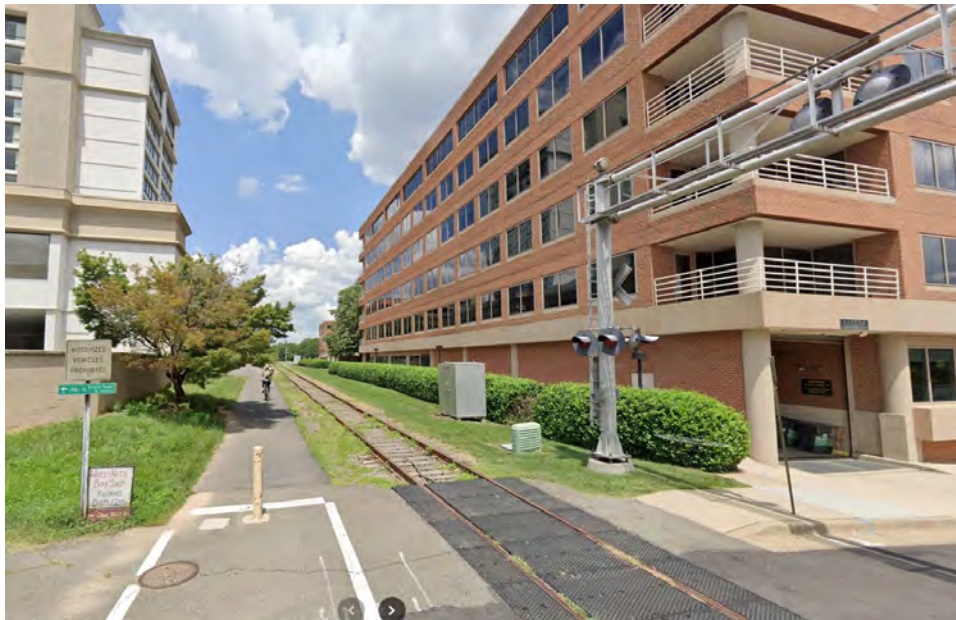
Figure 27: Mount Vernon Trail crossing Montgomery Street north of Old Town Alexandria, showing less than 6' separation between the trail and inactive rail line.
